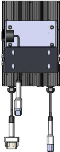
Once mounted, simply connect the alarm to the Relay Harness leaving the Antenna. It is the cable on the bottom-left in the Figure above.
